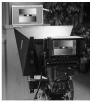
that they are color-matched and provide, as closely as is possible, the same picture. We use a chip-chart (*left*) to calibrate the cameras while viewing and comparing their output on a vector scope (*below*). This gives us a baseline for our cameras output and any adjustments that will be needed for the day. These two pictures illustrate this process.
